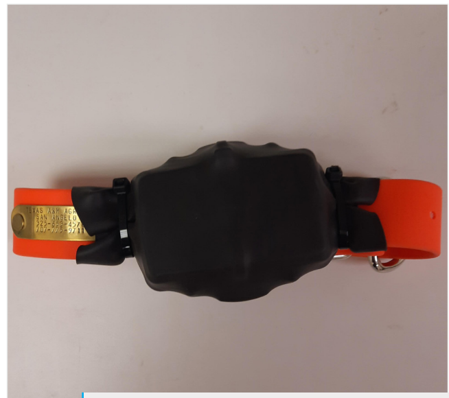
Oyster 3 GPS tracker attached to a 2 inch wide dog collar with electrical heat shrink and 3 zip ties.
