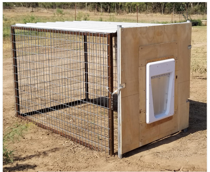
Figure 13. Aggie LGD Feeding Station with RFID door. (Photo courtesy of Texas A&M AgriLife, Costanzo 2018)
