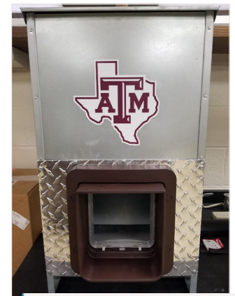
Figure 12. Aggie LGD RFID Feeder. (Photo courtesy of Texas A&M AgriLife, Costanzo 2018)
